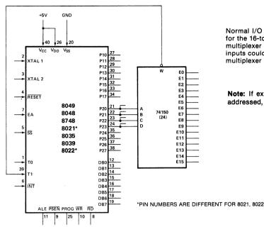
Normal I/O port is used to select an address for the 16-to-1 multiplexer. The output of the multiplexer is brought into a test input. Eight inputs could be added with a 74LS151 8-to-1 multiplexer using the same structure.
